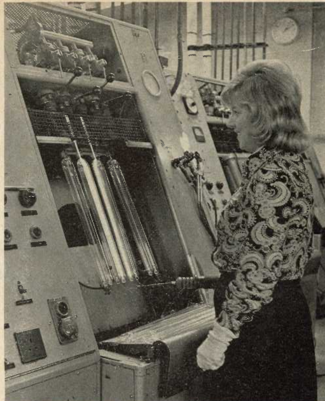
Left: Admitting the sodium to the lamp
